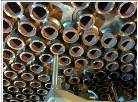
Figure 16: welding the new TTS joints
